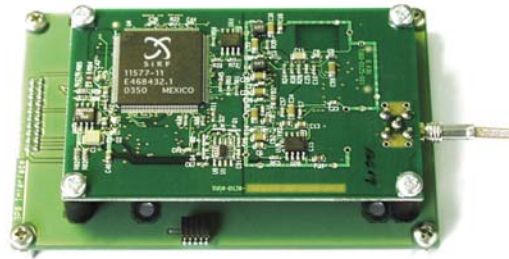
Figure 3 – Installing Navman Jupiter-T on the GPS Interface Board
