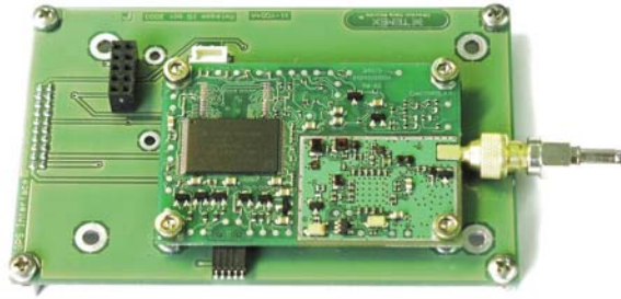
Figure 5 – Installing Motorola M12+ Timing on the GPS Interface Board
