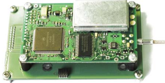
Figure 1 – Installing Motorola UT+ Oncore on the GPS Interface Board
